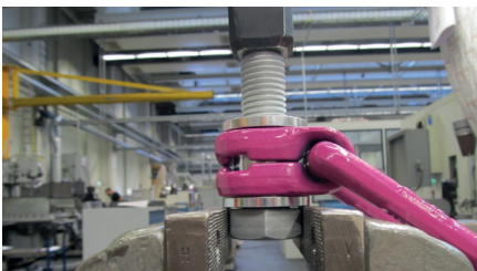
Pic. 8: Dismantling position of the VLBG-PLUS
